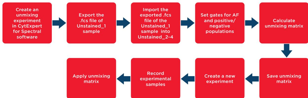
**Figure 1:** The process of spectral unmixing and autofluorescence (AF) extraction followed in this experiment using the CytoFLEX mosaic Spectral Detection Module.
